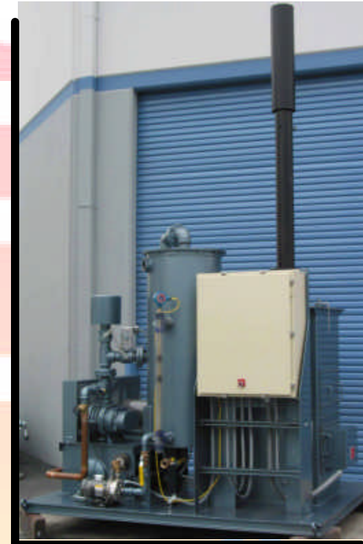
250 SCFM Electric Catalytic Oxidizer w/ Positive Displacement Pump Package
