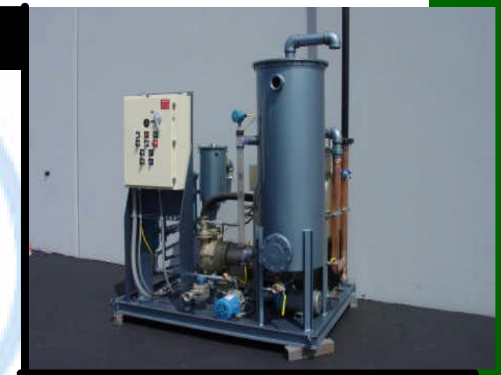
300 ACFM High Vacuum/Dual Phase Extraction System w/ Liquid Ring Pump
